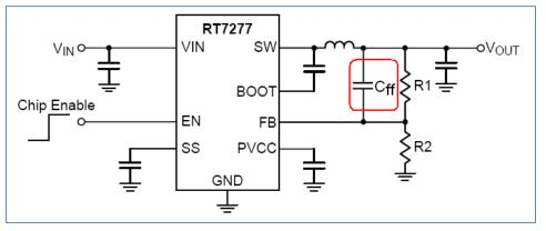
FIGURE 6: ACOT™ CONVERTER SCHEMATIC. FEED-FORWARD CAPACITOR C<sub>FF</sub> CAN BE USED TO INCREASE SYSTEM DAMPING
