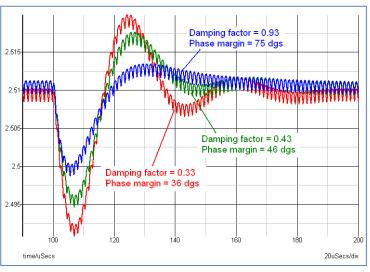
Figure 10 at the left shows a buck converter output voltage fluctuation during a fast load step transient with differing damping factors ( $\xi$ ).
