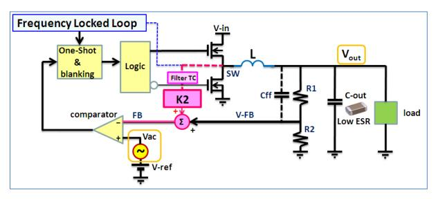
FIGURE 3: CLOSED LOOP MEASUREMENT OF ACOT BUCK CONVERTER
