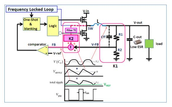
FIGURE 1: ACOT BUCK CONVERTER CONTROL MECHANISM AND OPERATION
