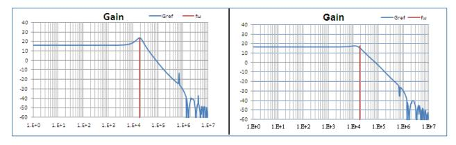
FIGURE 9: CLOSED LOOP GAIN WITHOUT CFF (LEFT) AND WITH CFF = 68PF (RIGHT)
