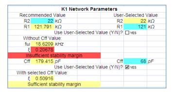
Figure 8: Calculation of the feedback network and damping factor  $\xi$  without and with C<sub>ff</sub>. Optimal value for C<sub>ff</sub> is 180pF, which will result in a damping factor > 0.707. When using C<sub>ff</sub> = 68pF, the damping factor will be 0.509, which is slightly under-damped condition, but provides sufficient stability margin.
