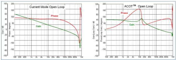
FIGURE 2: OPEN LOOP GAIN/PHASE SIMULATION OF CURRENT MODE AND ACOT CONVERTERS SHOW VERY DIFFERENT RESULTS
