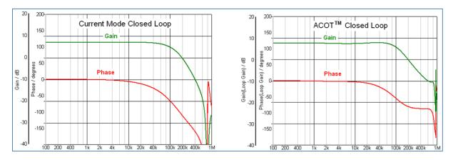
FIGURE 4: CLOSED LOOP GAIN/PHASE SIMULATION OF CURRENT MODE AND ACOT CONVERTERS SHOW SIMILAR GAIN AND PHASE CURVES
