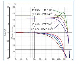
In closed loop mathematical analysis, the system stability can be found by observing the closed loop response. Flat gain response is considered stable (critically damped or over-damped response), while severe peaking in the gain with abruptly decreasing phase around resonance frequency (under-damped response) corresponds to low phase margin in the system open loop gain. See figure 5: Examples of Closed Loop gain/phase with various damping factors.
